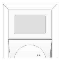
**5N module** - The illuminated window, 68mm wide, 40mm high, is suitable for entering address information, dialling information or name list (app. 15 in total). The backlight is powered by 12VAC (unit terminals: 12VAC), or 15VDC DC (unit terminals: +DC (+ ELOCK) and GND (- LINE).
