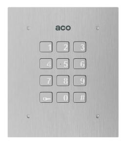
The autonomous INS–ZS code lock is a microprocessor device which serves the purpose of controlling one or two outputs independently, by means of the proper code for the given output. The outputs may control outdoor devices e.g. an electric door strike, reversible electric striker (only output 1) or optional relay, with which we can control any other device, e.g. an electromagnetic jumper, barrier, etc.
