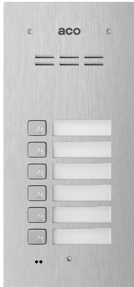
**IMPORTANT!** When disinfecting panels made of stainless steel, use only alcohol-based cleaners. All types of chlorides (which are present in the composition of common cleaners) are harmful to the steel surface, because they abrade its natural protective coating and increase the risk of corrosion marks.
