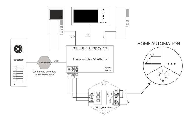
The module features screw connectors to connect the wires and is of a miniature size (diameter 50mm), hence it can be installed, for instance, in a standard 60 mm junction box. It can be plugged in anywhere in the installation and its location is in no way related to the receiver supported by it. Connect the module to the bus at any location by plugging the wires into the appropriate terminals: **LINE** (audio signal), **+DC POWER** and **-DC POWER** (power supply).
