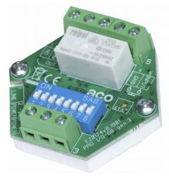
The PRO I/0-60 (G3) module is an optional extension module for the PRO system; it is used as a control module for home automation and external devices, additional signalling and autoopening. Designed for installation in Ø60mm junction box. PRO I/0-60 (G3) is compatible with all COMO/ Familio PRO, PRO-A devices.
